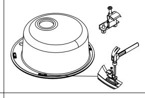
5 Put a bead of Sealant around the top edge of cutout to seal the Sink/Basin to the Worktop and to stop water from Leaking into your cupboard.
