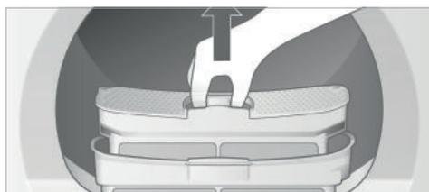
Remove inner filter **A** and flip it open.
