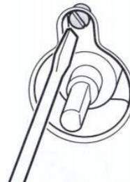
Turn on the burners respectively after conversion and remove the button on the control panel and set the flame length by tightening or loosening the screw on the gas valve (12.4 cock) or in the valve shaft.
