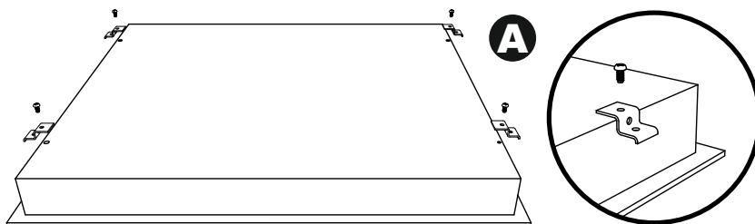
**Attention!** To install the appliance is not recommended the use of the silicone or other sealants and other adhesives besides the supplied mounting materials. If additional fastening materials and substances have been used, the removing the device from the mounting niche in case of necessary service is provided by and at the expense of the owner. The manufacturer and the customer services are not responsible for damages of equipment and furniture because of the disassembling.
