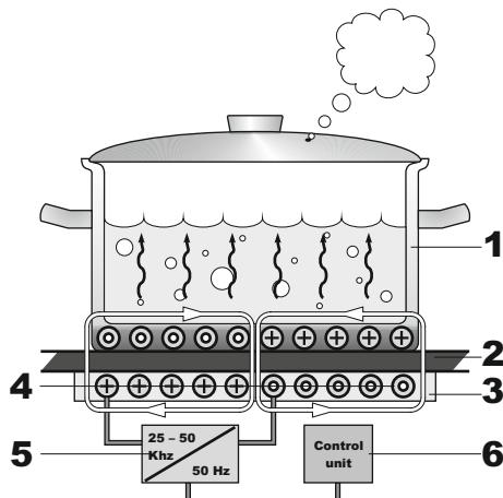
1. Utensil made of ferromagnetic material
