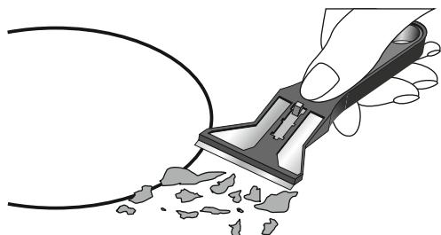
Pieces of aluminum foil and plastic material which have inadvertently melted or sugar remains or highly sacchariferous food have to be removed immediately from the hot cooking area with the special scraper to avoid any possible damage to the surface of the top.
