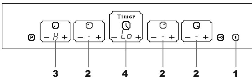
After switching-ON the electronic control remains activated for 1 minute. If no cooking zone or timer selection follows within this period of time, the electronic control automatically switches off.
