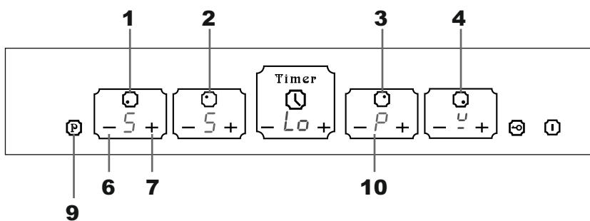
The display of the corresponding cooking zone shows a symbol **10**, **P**. The function **Power** is activated.
