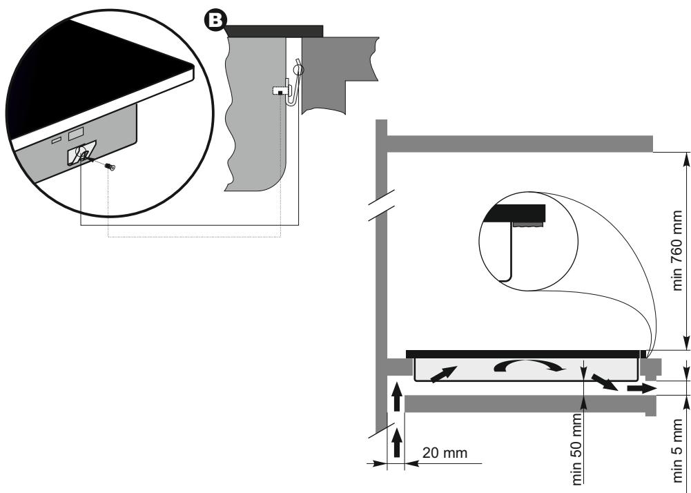
**Attention!** Installation and electrical connection of the cooking hob must be made by a qualified expert only.
