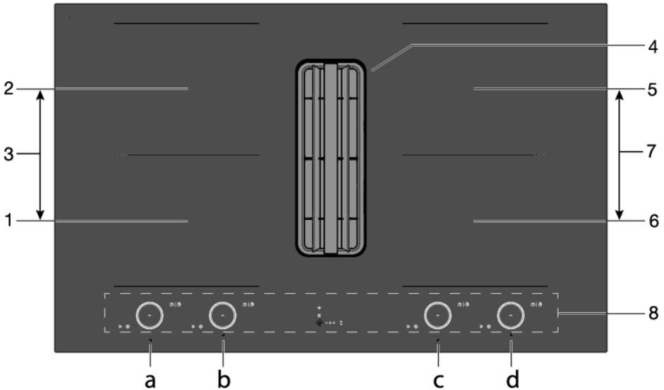
1. Bridge Induction Cooking zone 18 x 22 cm / max. 2.3 kW / max. 3.7 kW (boost) to be operated with 'a'
