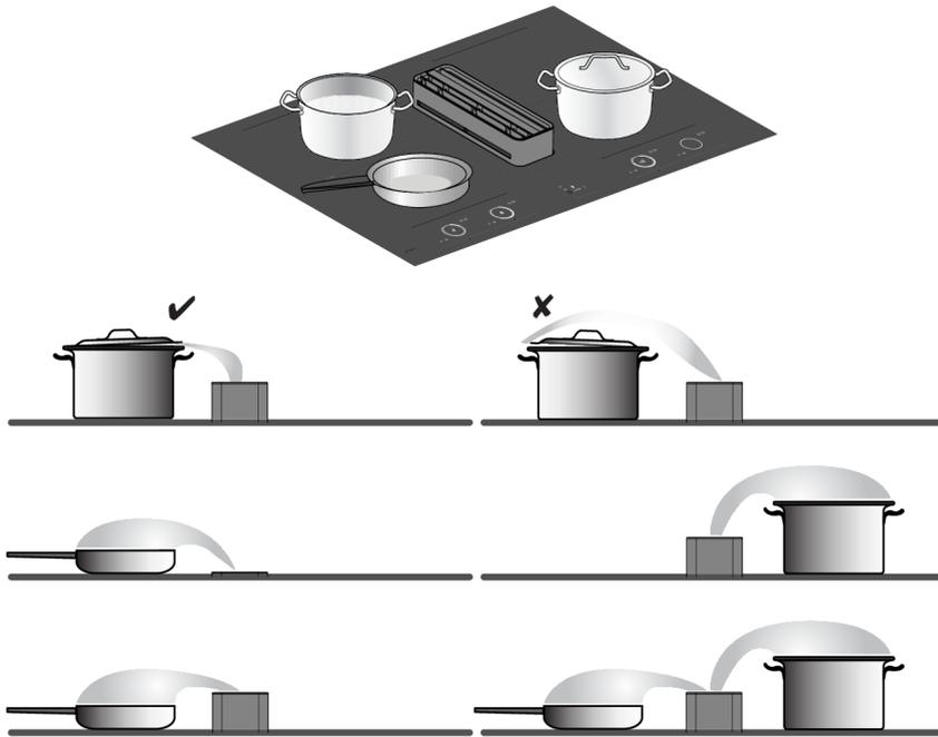
We recommend placing pans as close to the tower as possible, within the dimensions of the cooking zones. If a lid is used, place it at an angle on the pan with the opening towards the tower. This ensures optimal extraction.
