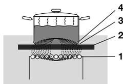
The coil (1) in the hob (2) generates a magnetic field (3). By placing a pan with an iron base (4) on the coil, a current is induced in the base of the pan.
