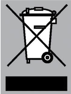
The product has been marked with a crossed-out dustbin symbol to remind you of the obligation to dispose of electrical household appliances separately. This means that the appliance may not be included with normal domestic refuse at the end of its service life. The appliance must be taken to a special municipal centre for separated waste collection or to a dealer providing this service.
