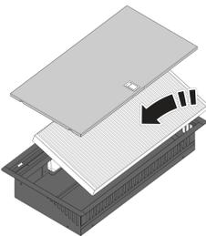
The recirculation box with a filter is located under the bottom of the cabinet and is accessible from the kitchen cabinet.
