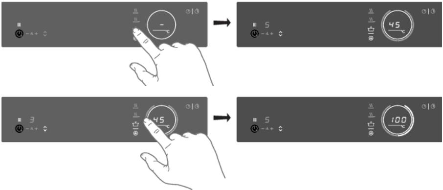
When the program or temperature selection does not change for 3 seconds, the program is activated. To deactivate a PLUS program, press the active program key for about three seconds or select a power level manually.
