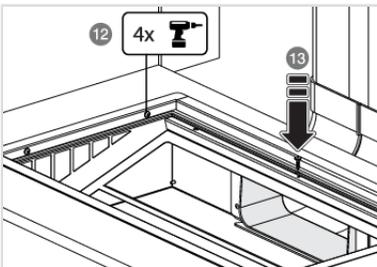
12. Remove the cover of the box and screw the box in place from the inside.
