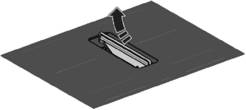
When indicated by the filter indicator, the metal filters must be cleaned by hand or in the dishwasher at low temperatures with a short program. Never put the plastic frames in the dishwasher separately, without metal grease filters. See chapter 'Settings' for filter cleaning settings.
