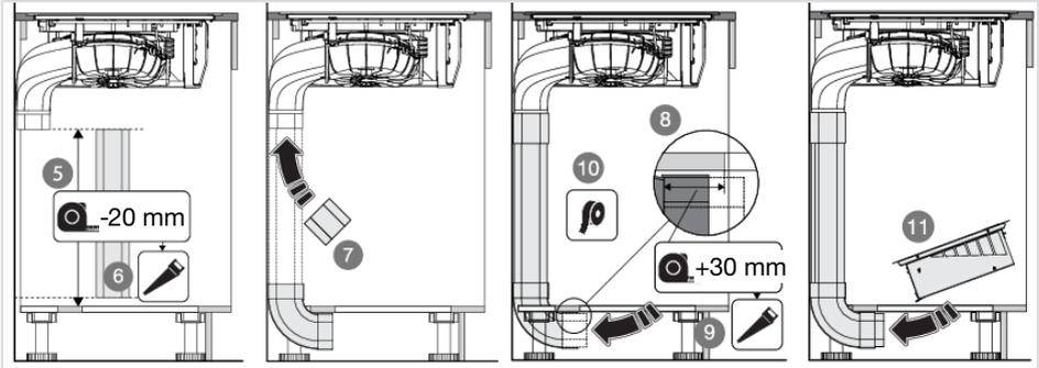
5. Measure the distance as indicated in the figure and subtract 20 mm.
