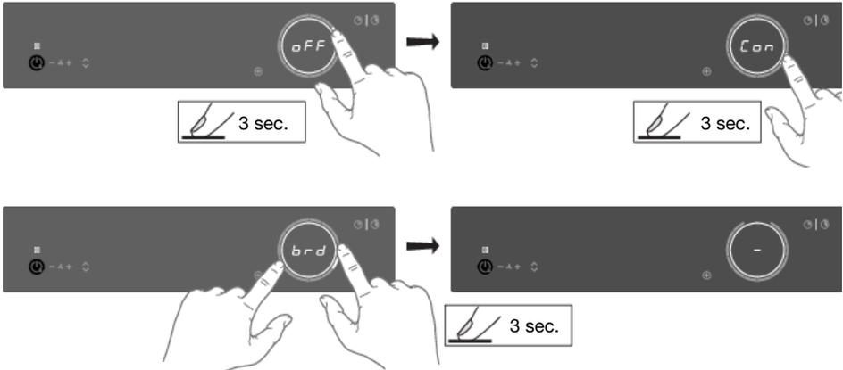
To exit the menu, touch with two fingers anywhere the slider for 3 seconds.
