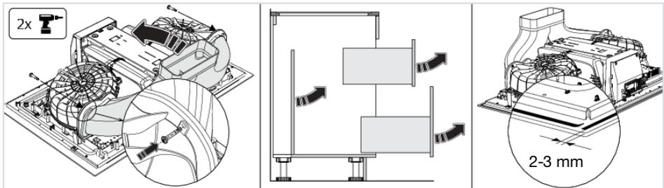
1. Hook the Y-duct into the lower edge of both motor housings and tilt the Y-duct up.
