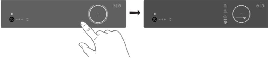
2. Select the desired program and temperature range by touching the relevant symbol. You can also toggle through the menu or temperature by long-pressing the relating touch key.
