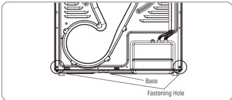
4. Adjust the height of the four feet of the dryer so that the height limit plugs of the feet can just be inserted, and the height is about 11.5 mm.
