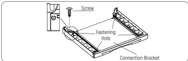
3. Remove the bottom 2 screws on both sides of the back of the dryer and set it aside for later use.
