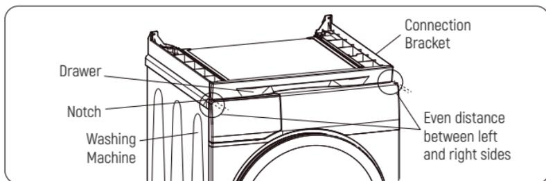
2. Fix the connecting bracket and the top cover of the washing machine with 4 Tapping Screws.
