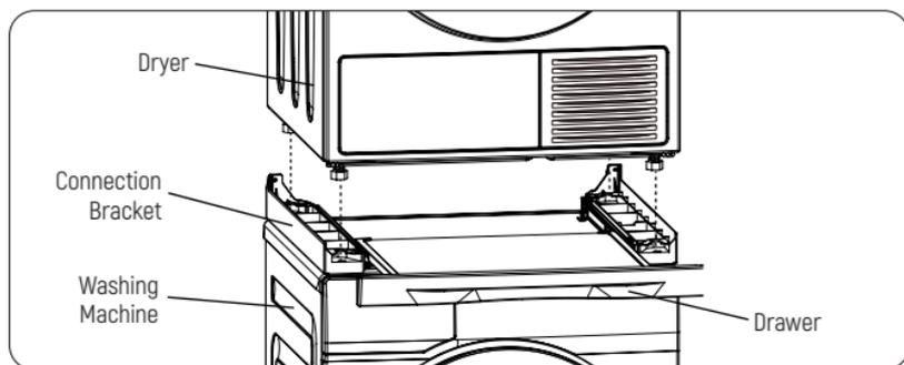
7. Take the 2 screws that were removed just now, pass the screws through the screw holes connecting the bracket and the lower part of the rear panel of the dryer, and then fasten them in place.
