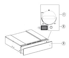
The control elements are the temperature knob and the luminous ON-OFF switch.
