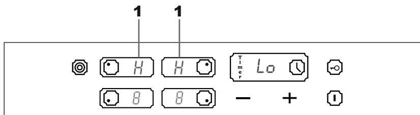
If you didn't turn off one or several cooking zones after use the hob, then they will turn off automatically after elapsing a maximal working time one of them. In this case the indicators of the corresponding zones **1** show symbols **H**.
