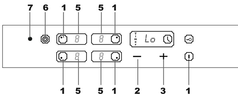
The indicator **7** lights up. It comes a sound signal. The bigger heating elements are heated to the level chosen for the smaller element.
