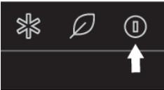
1. Touch the On/Off key for three seconds.
