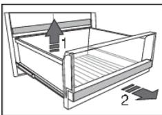
A number of drawers are mounted on fully extending telescopic rails and are fitted with a soft-close system.
