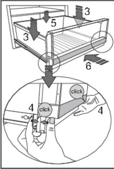
To fit the drawer onto the rails, pull the two rails fully out. Place the drawer on the rails (3). In the front, press the drawer and the rails towards each other on the right and the left side until you hear a “click” (4). Press the back of the drawer downwards if necessary (5). Finally, slide the drawer on the rails fully in (6).
