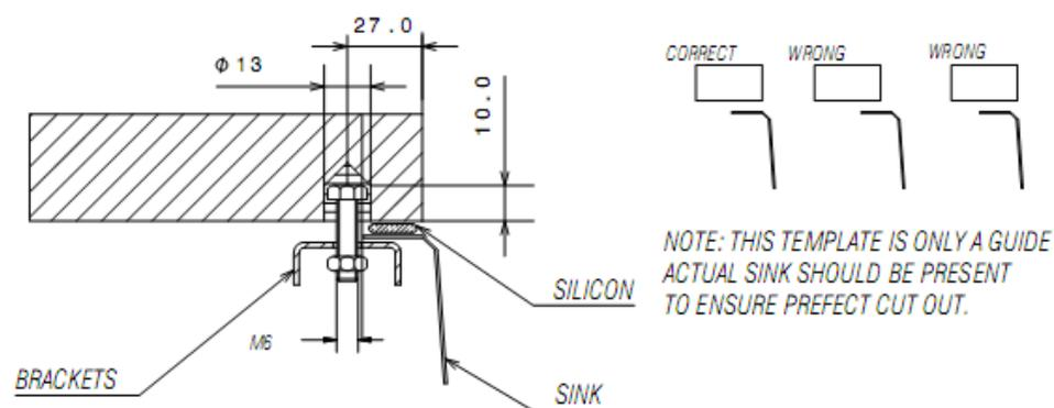
2) Determine placement of clip brackets. Pre-drill holes according to method desired based on countertop material.
